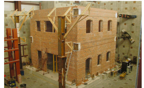
Full-scale testing of unreinforced masonry building.
