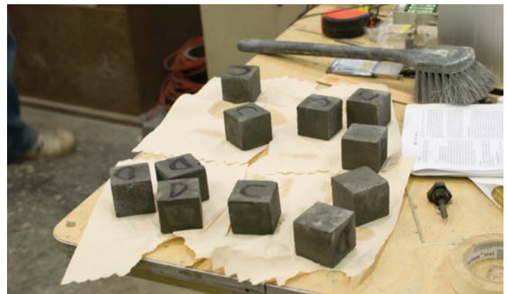
Concrete bricks made with coal fly ash. Different mixtures are tested for their weight and tensile strength.
